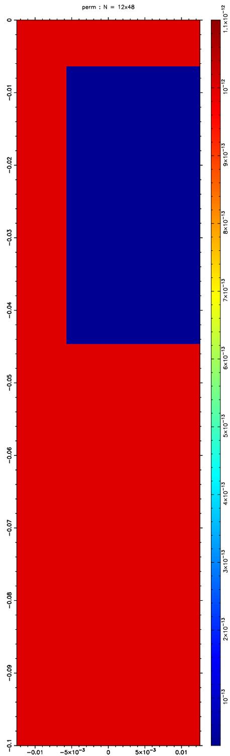
Fig. 9 Pattern for the simulation. Due to symmetry, only the half of the square blocks is considered. Dirichlet condition is applied on the top, whereas Neumann condition is applied to others.
