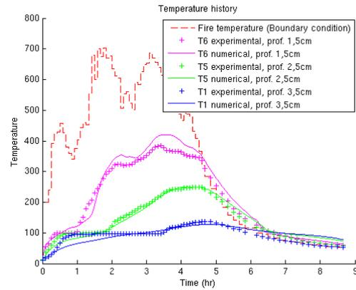
**Fig. 3** Comparison between numerical results and experimental data (realized on the archaeological hearths at Pincevent site; a real fire has been used).
