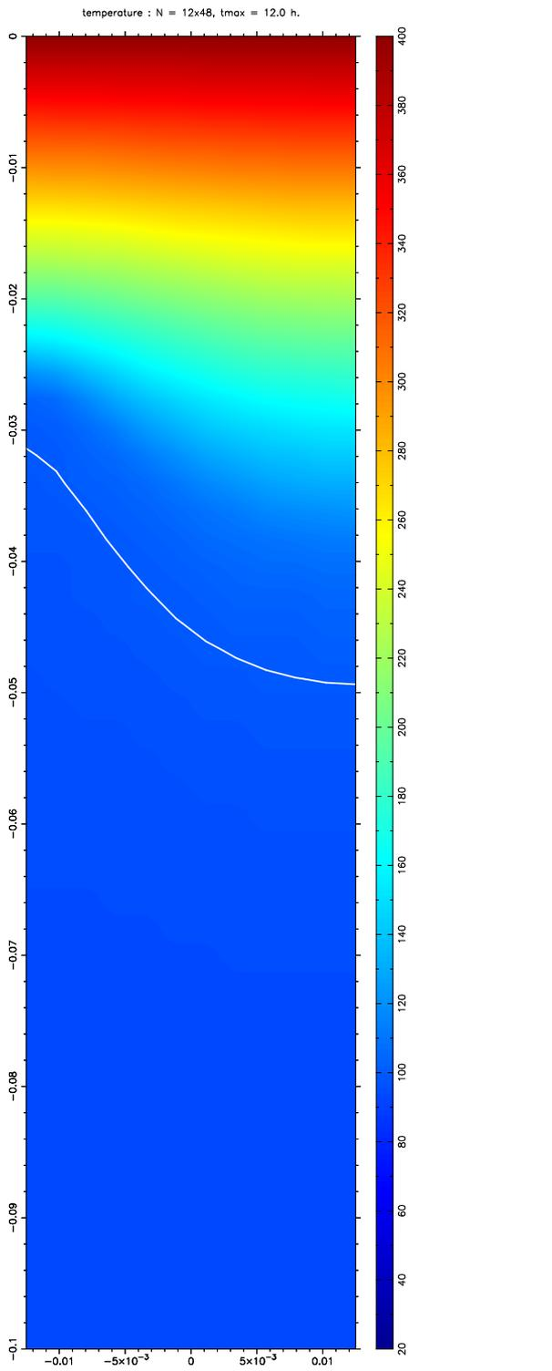
Fig. 8 Temperature field. Phase-change interface is shown by the white line.
