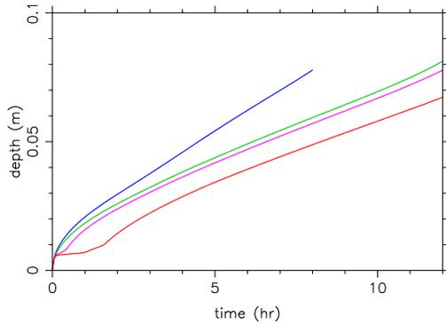
**Fig. 4 Phase-change interface position for different cases: (blue) heating without coupling, (green) homogeneous permeability, (magenta) weak difference in permeability and (red) strong difference.**
