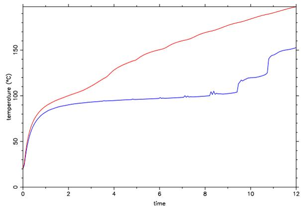
**Fig. 6 Temperature evolution for two fixed sensors, when the soil is constituted by two vertical blocks: each curve has the same color as the corresponding block.**
